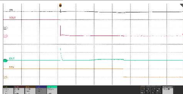
Figure 6-34. Transient Overcurrent Blanking Timer Response
