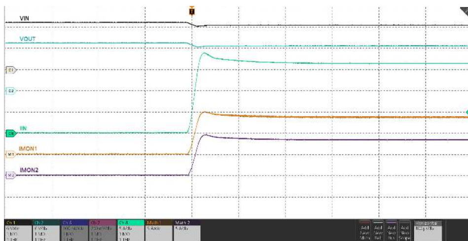
Figure 8-4. Parallel Devices Load Current During Steady-State
