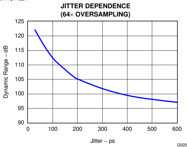
Figure 38. Jitter Sensitivity
