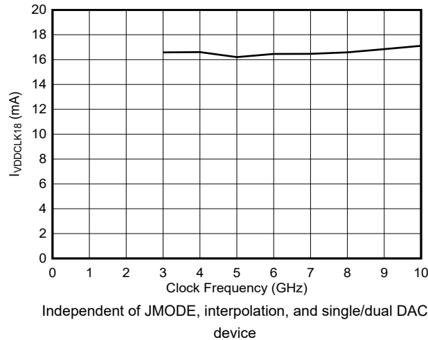
Figure 6-217. VDDCLK18 Current vs Clock Frequency
