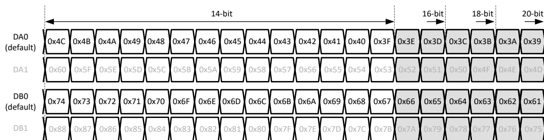
Figure 8-38. 1-wire output bit mapping
