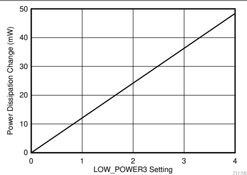
Figure 6-13. Power Dissipation Change vs LOW_POWER3 register setting
