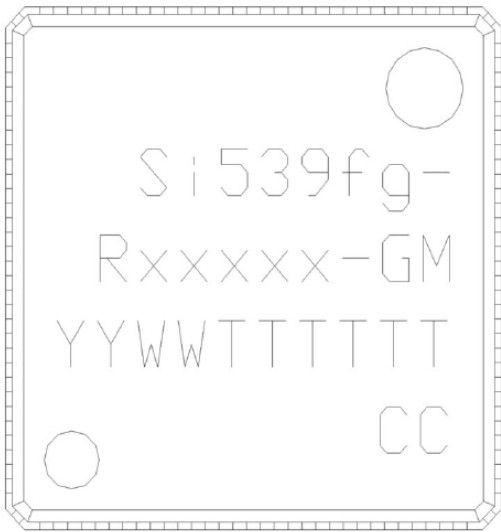
Figure 34. Si5396C/D and Si5397A/B/C/D QFN 9x9 mm Package
