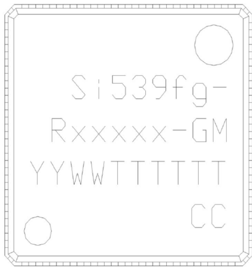
Figure 34. Si5396C/D and Si5397A/B/C/D QFN 9x9 mm Package
