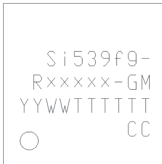
Figure 39. Si5392 and Si5394 A/B/C/D/P QFN 7x7 mm Package, Si5392 and Si5394 J/K/L/M/E - LGA 7x7 mm Package, Si5395J/K/L/M/E - LGA 9x9 mm Package
