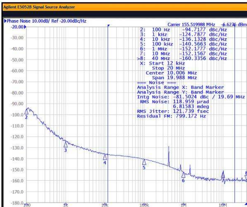
Figure 8.3. Input = 25 MHz; Output = 155.52 MHz, 2.5 V LVDS
