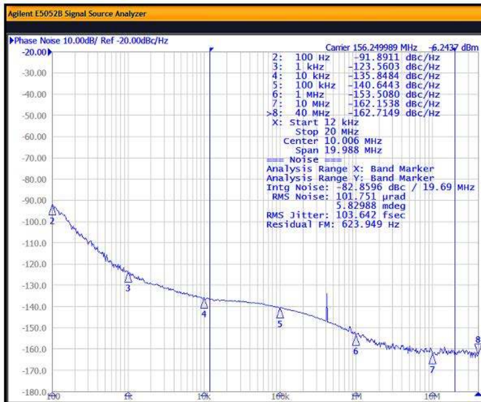
Figure 8.2. Input = 25 MHz; Output = 156.25 MHz, 2.5 V LVDS
