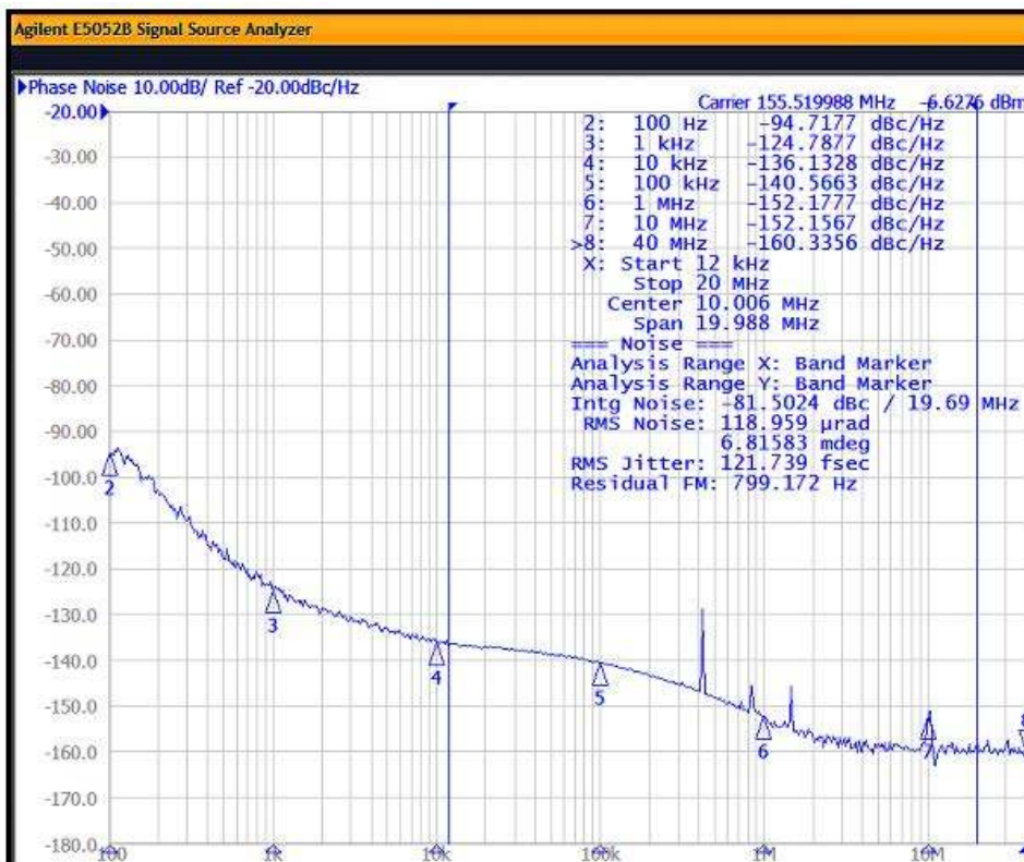
Figure 8.3. Input = 25 MHz; Output = 155.52 MHz, 2.5 V LVDS
