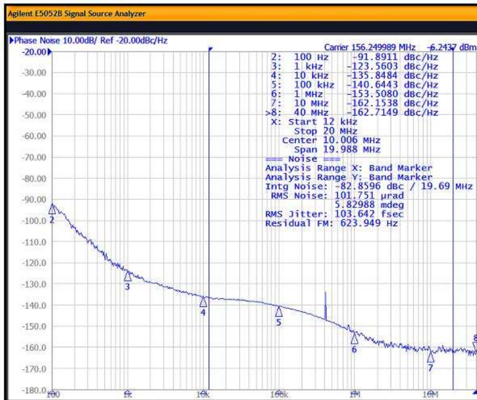
Figure 8.2. Input = 25 MHz; Output = 156.25 MHz, 2.5 V LVDS
