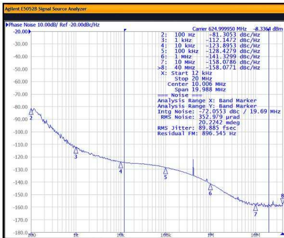
Figure 8.1. Input = 25 MHz; Output = 625 MHz, 2.5 V LVDS
