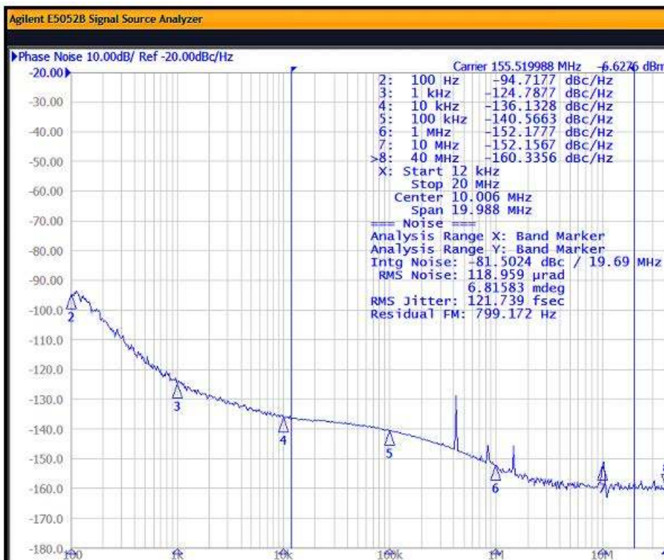
Figure 8.3. Input = 25 MHz; Output = 155.52 MHz, 2.5 V LVDS
