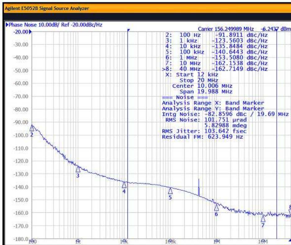
Figure 8.2. Input = 25 MHz; Output = 156.25 MHz, 2.5 V LVDS
