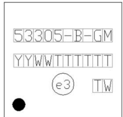
Figure 8.6. Si53305 Top Marking
