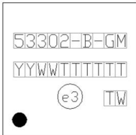
Figure 8.4. Si53302 Top Marking
