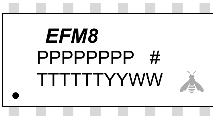
Figure 8.3. SOIC16 Package Marking
