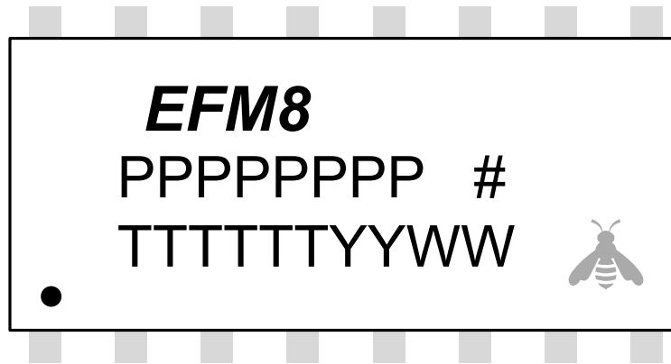
Figure 9.3. SOIC16 Package Marking
