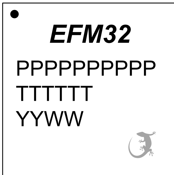
Figure 7.3. BGA125 Package Marking
