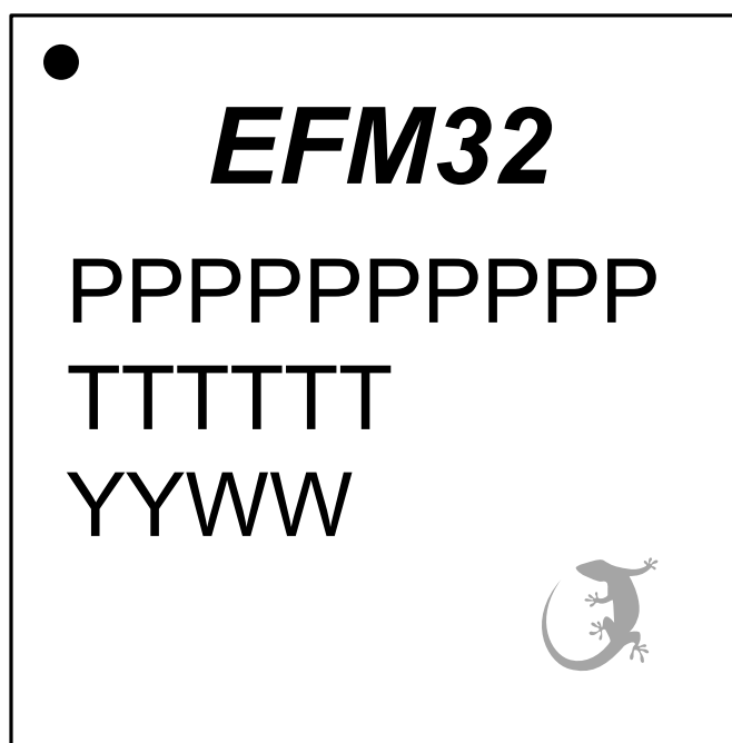
Figure 8.3. TQFP100 Package Marking
