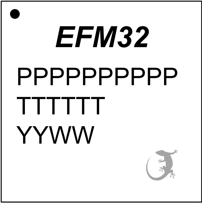
Figure 10.3. TQFP100 Package Marking
