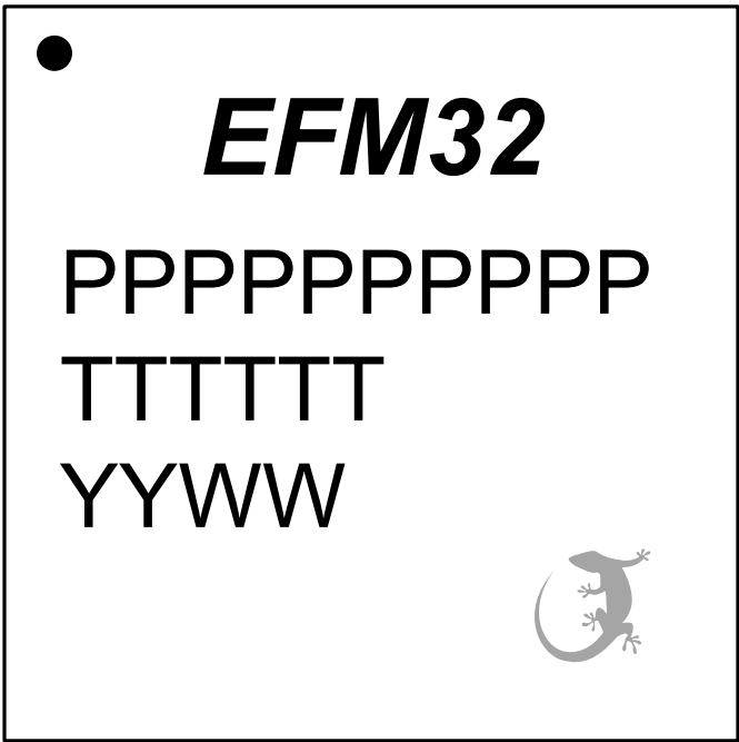
Figure 10.3. TQFP100 Package Marking
