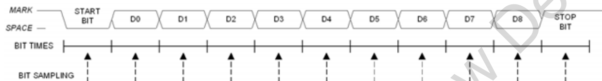
Figure 25.5. 9-Bit UART Timing Diagram
