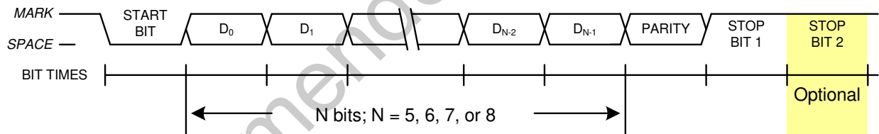
Figure 24.3. UART1 Timing With Parity
