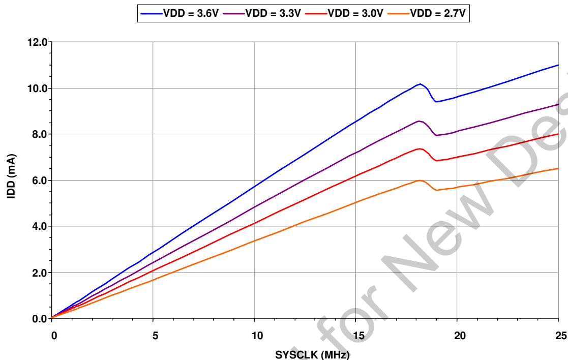
Figure 6.1. Normal Mode Digital Supply Current vs. Frequency
