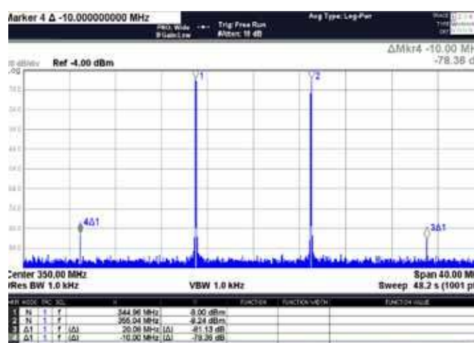
Fig 12. IMD3 (dBc) for two tones (spacing 10 MHz) centered at 350 MHz
