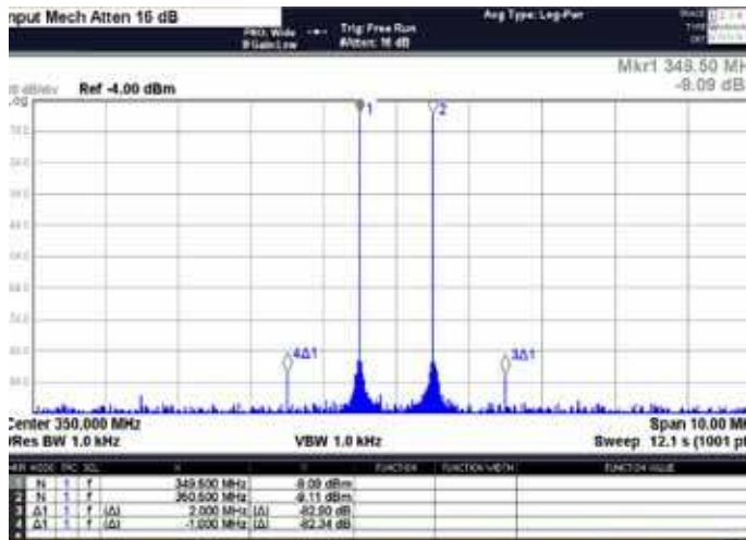
Fig 11. IMD3 (dBc) for two tones (spacing 1 MHz) centered at 350 MHz
