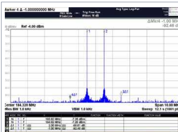
Fig 9. IMD3 (dBc) for two tones (spacing 1 MHz) centered at 184.32 MHz
