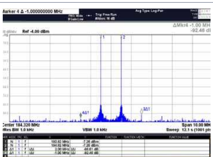
Fig 10. IMD3 (dBc) for two tones (spacing 10 MHz) centered at 184.32 MHz
