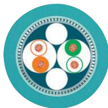
PUR ETHERNET 2x2 FLEX [93E]
