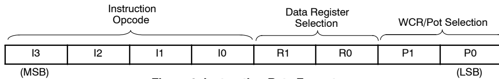
Figure 9. Instruction Byte Format
