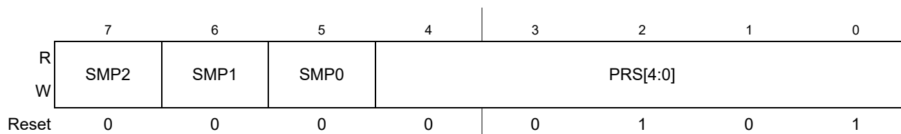
Figure 14-7. ATD Control Register 4 (ATDCTL4)
