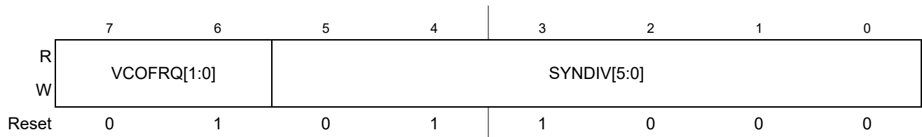
Figure 10-4. S12CPMU Synthesizer Register (CPMUSYNR)
