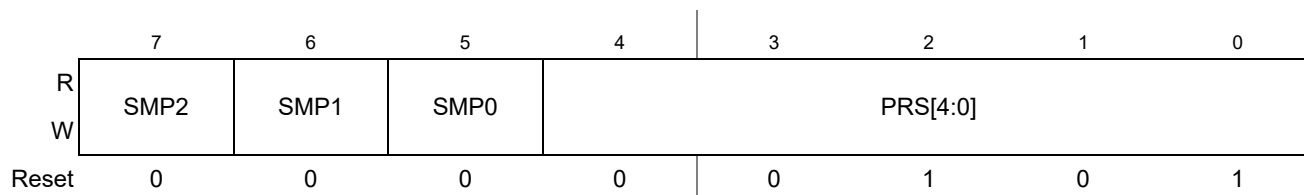
Figure 15-7. ATD Control Register 4 (ATDCTL4)
