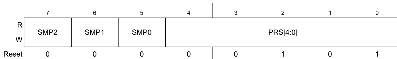
Figure 13-7. ATD Control Register 4 (ATDCTL4)
