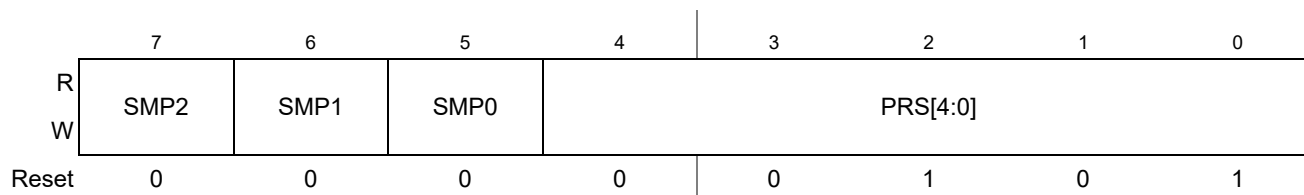
Figure 11-7. ATD Control Register 4 (ATDCTL4)
