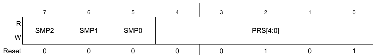
Figure 12-7. ATD Control Register 4 (ATDCTL4)
