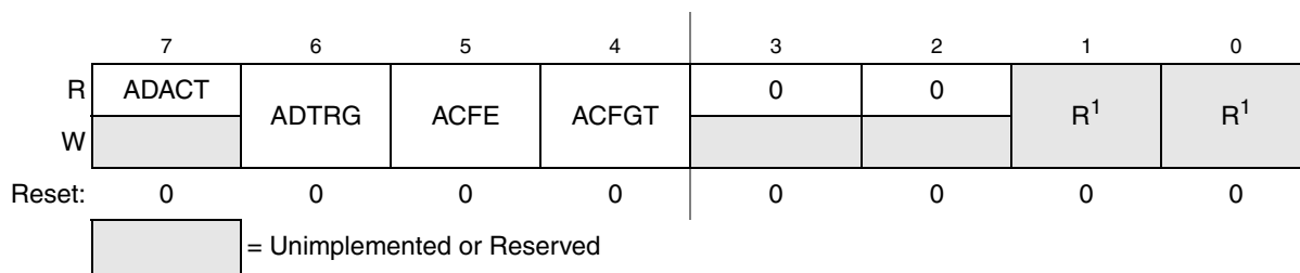
Figure 9-5. Status and Control Register 2 (ADCSC2)
