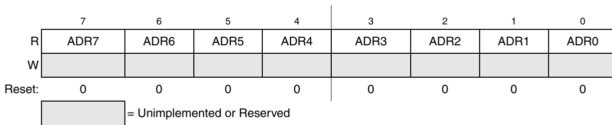
Figure 8-7. Data Result Low Register (ADCRL)
