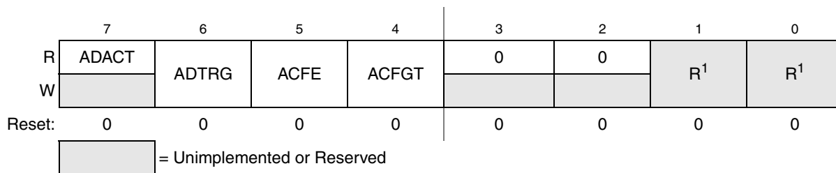
Figure 8-5. Status and Control Register 2 (ADCSC2)
