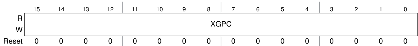
Figure 6-10. XGATE Program Counter Register (XGPC)
