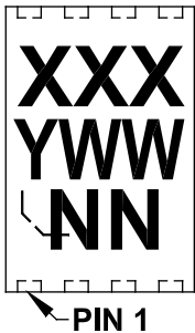
8-Lead DFN (2x3x0.9 mm) 8-Lead UDFN (2x3x0.5 mm)
