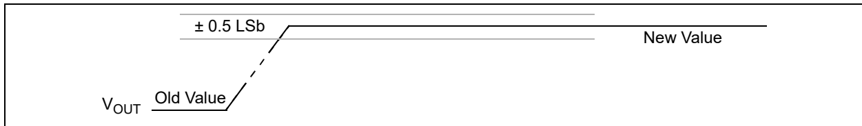
FIGURE 1-1: V_{OUT} Settling Time Waveforms.
