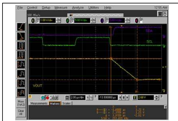
FIGURE 2-99: Half-Scale Settling Time (C00h to 400h) (MCP4726).
