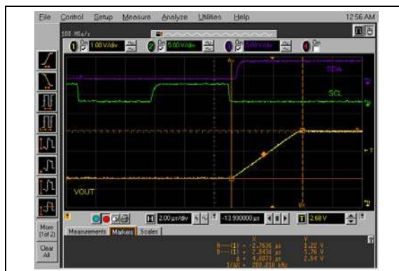
FIGURE 2-98: Half-Scale Settling Time (400h to C00h) (MCP4726).
