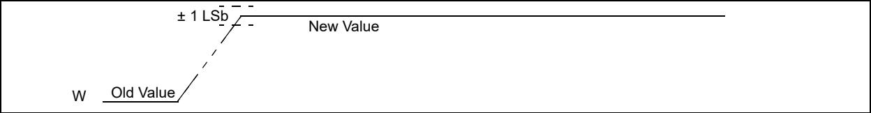
FIGURE 1-1: Settling Time Waveforms.
