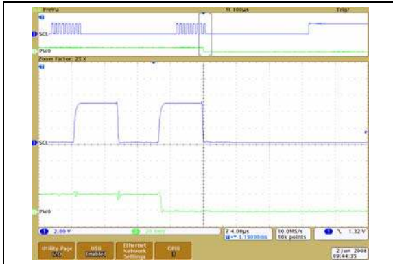
FIGURE 2-63: 100 k \Omega – Low-Voltage Decrement Wiper Settling Time ( V_{DD} = 2.7\text{V} ) (1 \mu\text{s}/\text{Div} ).
