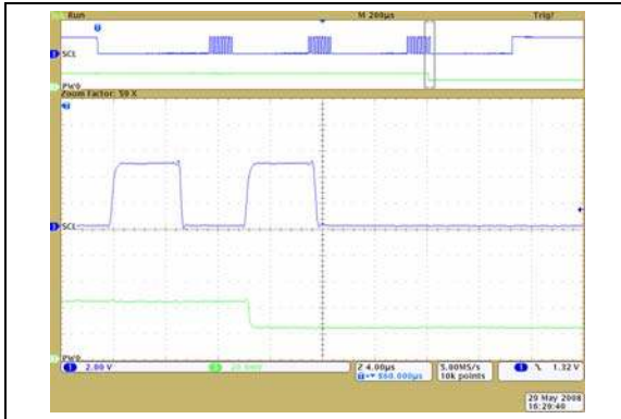
FIGURE 2-33: 10\text{ k}\Omega – Low-Voltage Decrement Wiper Settling Time ( V_{DD} = 2.7\text{V} ) ( 1\text{ }\mu\text{s}/\text{Div} ).
