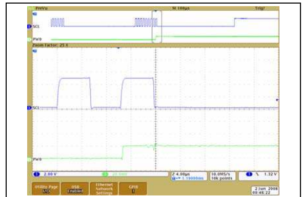
FIGURE 2-66: 100 k \Omega – Low-Voltage Increment Wiper Settling Time ( V_{DD} = 5.5\text{V} ) (1 \mu\text{s}/\text{Div} ).
