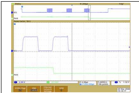
FIGURE 2-49: 50 k \Omega – Low-Voltage Decrement Wiper Settling Time ( V_{DD} = 5.5\text{V} ) (1 \mu\text{s}/\text{Div} ).
