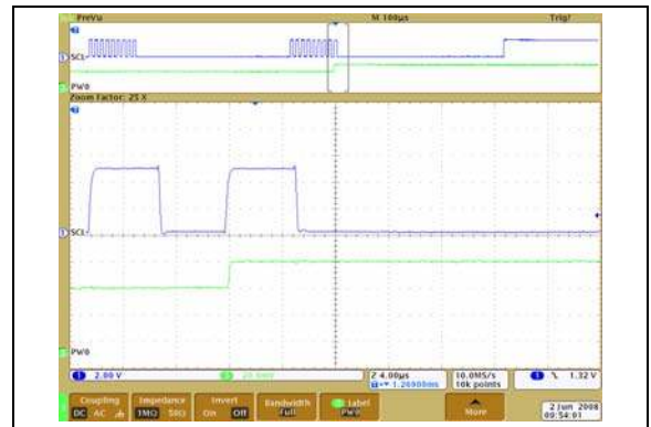
FIGURE 2-21: 5\text{ k}\Omega – Low-Voltage Increment Wiper Settling Time ( V_{DD} = 5.5\text{V} ) ( 1\text{ }\mu\text{s/Div} ).
