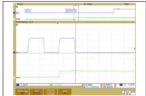
FIGURE 2-66: 100 k \Omega – Low-Voltage Increment Wiper Settling Time ( V_{DD} = 5.5\text{V} ) (1 \mu\text{s}/\text{Div} ).
