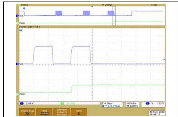
FIGURE 2-51: 50 k \Omega – Low-Voltage Increment Wiper Settling Time ( V_{DD} = 5.5\text{V} ) (1 \mu\text{s}/\text{Div} ).
