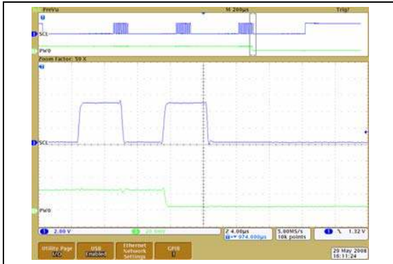
FIGURE 2-48: 50 k \Omega – Low-Voltage Decrement Wiper Settling Time ( V_{DD} = 2.7\text{V} ) (1 \mu\text{s}/\text{Div} ).
