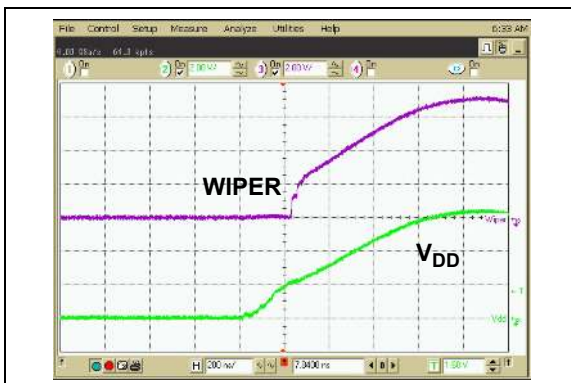
FIGURE 2-45: 50 kΩ – Power-Up Wiper Response Time.
