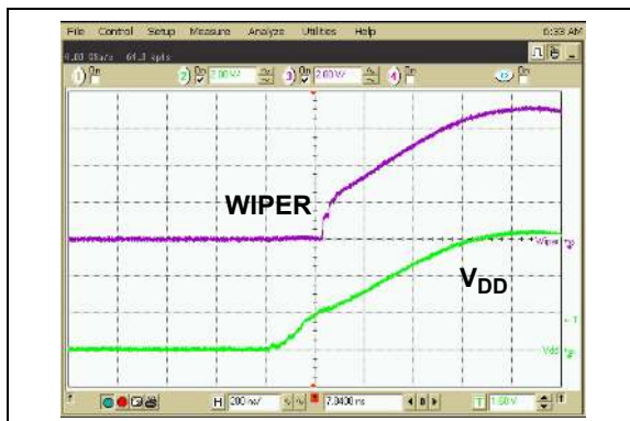
FIGURE 2-52: 50 k \Omega – Power-Up Wiper Response Time.
