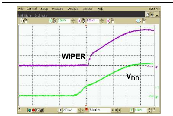
FIGURE 2-52: 50 kΩ – Power-Up Wiper Response Time.
