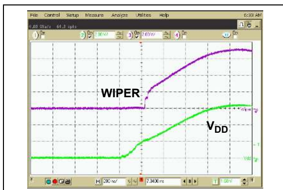
FIGURE 2-52: 50 k \Omega – Power-Up Wiper Response Time.
