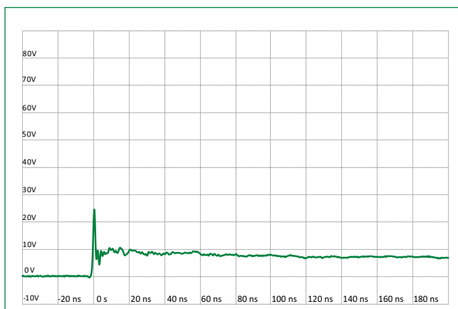
ISO10605 Contact Discharge Plot at +8 kV
