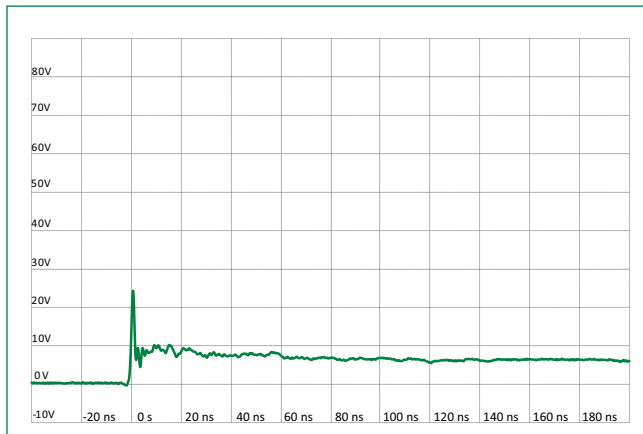
IEC 61000-4-2 +8 kV Contact ESD Clamping Voltage
